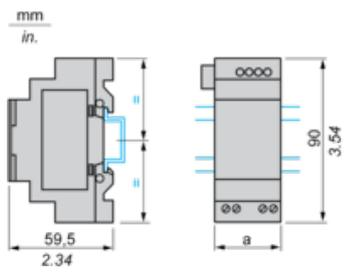
**Screw Fixing (Retractable Lugs)**
