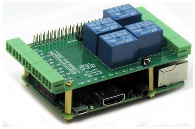
The 4-RELAYS-4-INPUTS card is a stackable expansion card for Raspberry Pi. It is compatible with all Raspberry Pi versions from Zero to 4. It offers a compact and inexpensive solution for adding up to 32 relays to your Raspberry Pi project. In addition, the card can read 4 optically isolated, digital inputs, ranging from 3V to 240V AC or DC.
