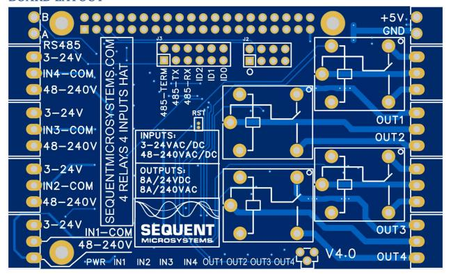
The 4-RELAYS-4-INPUTS card comes with appropriate mounting hardware. Up to eight cards can be stacked on top of one Raspberry Pi.
