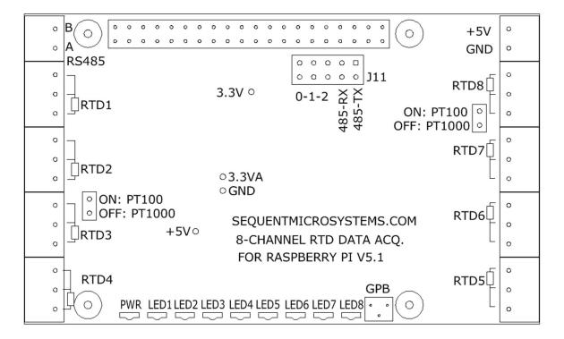
Your 8-Channels RTD Card comes with appropriate mounting hardware. Up to eight cards can be stacked on top of one Raspberry Pi. The power LED indicates when power is applied to the board. Each channel has one LED which can be programmed to turn on at the desired input threshold.
