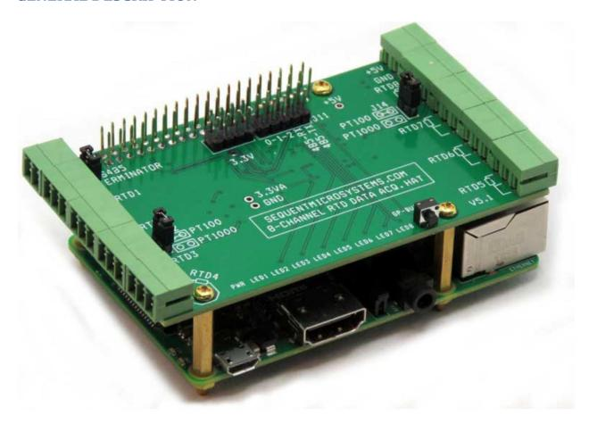
The 8-CHANNEL RTD Data Acquisition Card is a stackable expansion card for Raspberry Pi. It is compatible with all Raspberry Pi versions from Zero to 4 and offers a compact and inexpensive solution for reading and storing data from up to 64 RTD-100 temperature sensors.
