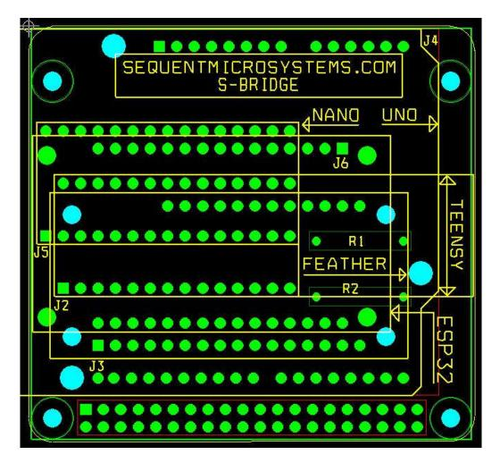
The Raspberry Pi Replacement card is an adaptor between any Raspberry Pi add-on card which used the I2C port for communication, and five of the most popular processor platforms in use today: UNO, NANO, TEENSY, FEATHER and ESP32.
