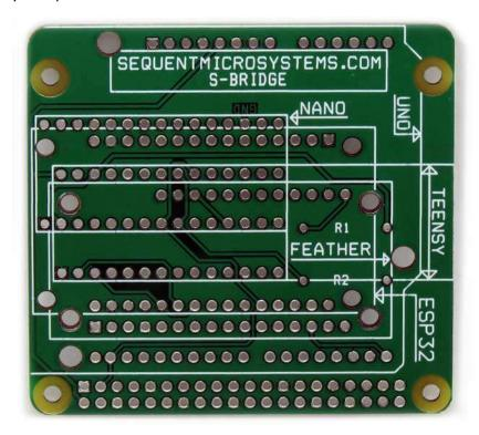
2. 2X20 male header (similar with Raspberry Pi GPIO connector).
