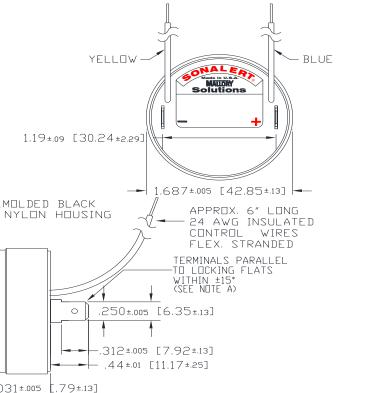
MOUNTING: REMOVE BLACK PLASTIC NUT AND INSERT THREADED FRONT THROUGH 1.25"
