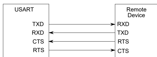
Figure 35-7. Connection with a Remote Device for Hardware Handshaking
