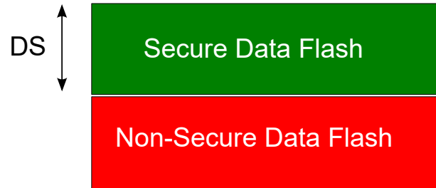
Figure 13-3. SAM L11 Data Flash Memory Mapping
