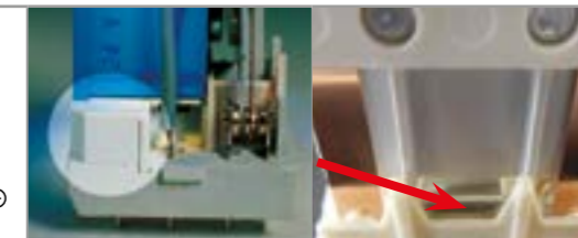
B: Contact circuit 5, 6 Additional physical separator between coil and contacts (for SELV applications)
