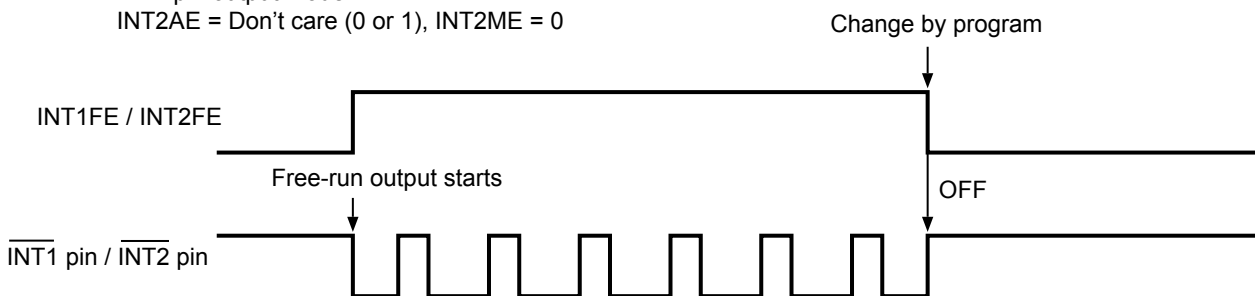
Figure 26 Output Timing of User-set Frequency
