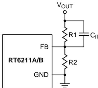
Figure 1. C<sub>ff</sub> Capacitor Setting
