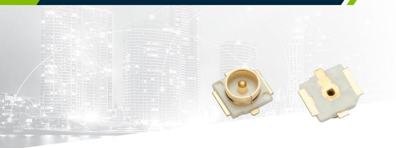
Part of the Taoglas SMD Mount Receptacle, the RECE.20279.001E.01 is a 3-pad type wire-to-board SMD receptacle that is ultra-small, lightweight and low profile, 2.5mm max. With an operational frequency range of DC to 6 GHz the RECE.20279.001E.01 is gold plated to provide superior performance and allow for ease of mounting with the male RF connector.
