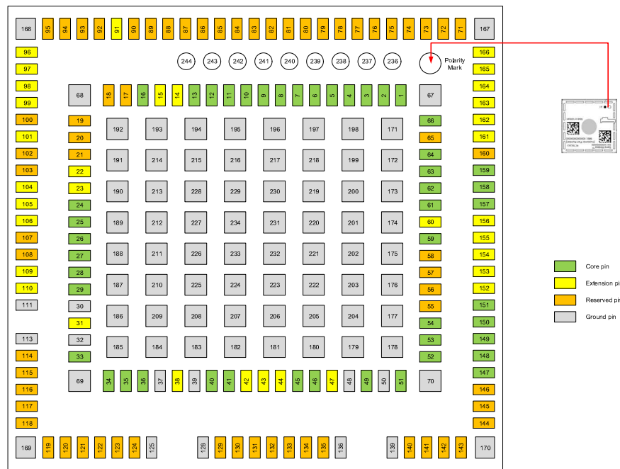
Figure 10-1: Pin Configuration (Top View, Through Module)
