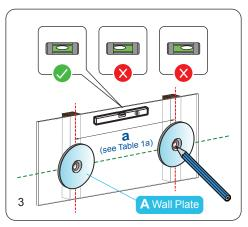
Using the wall plate (A) as a template, mark two holes for drilling on the centerline of the stud.
