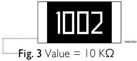
E24/E96 series: 4 digits, 1%, 0.5% First three digits for significant figure and 4th digit for number of zeros
