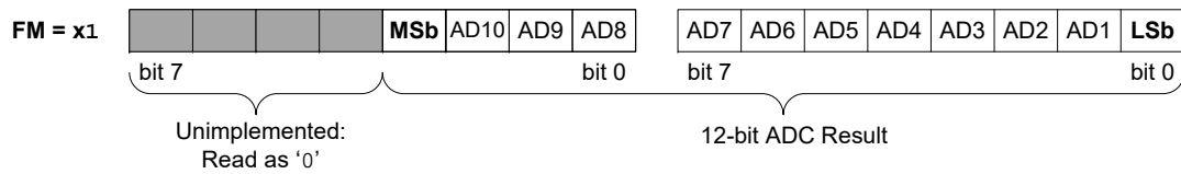
Figure 33-4. 12-Bit ADC Conversion Result Alignment/Format: IC = 0, FM = x1
