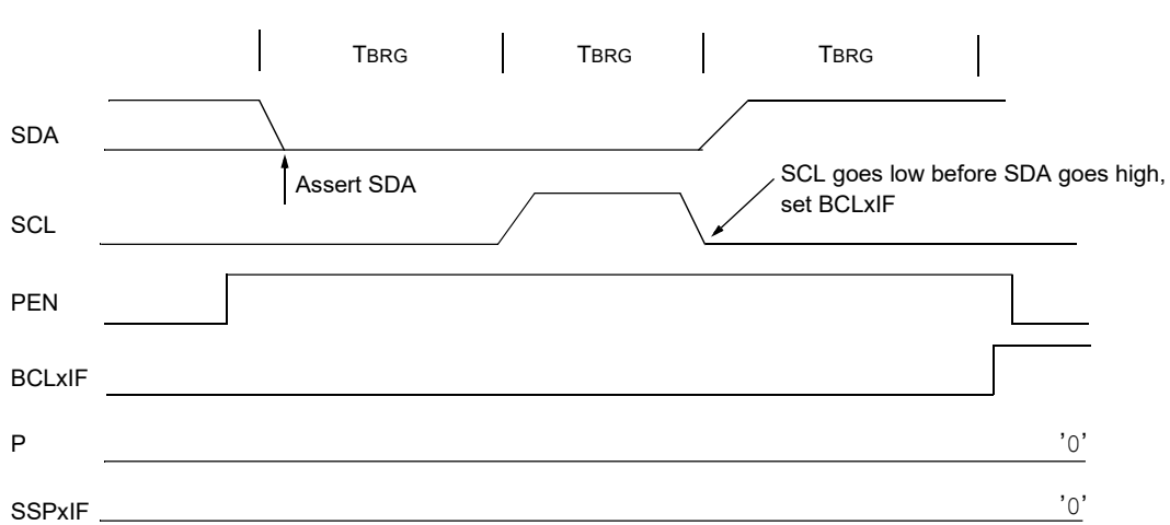
Figure 31-40. Bus Collision During a Stop Condition (Case 2)
