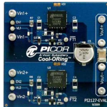
Figure 1: PI2127-EVAL1 Evaluation Board (1.8" x 1.8")
