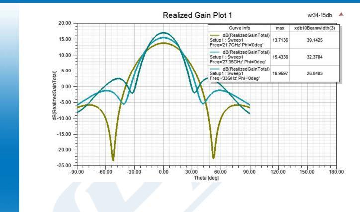
Click the following link (or enter part number in "SEARCH" on website) to obtain additional part information including price, inventory and certifications: WR-34 Standard Gain Horn Antenna Operating From 22 GHz to 33 GHz, 15 dBi Nominal Gain, UG-1530/U Flange PEWAN034-15
