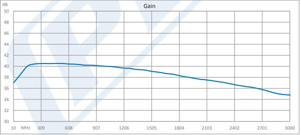
Click the following link (or enter part number in "SEARCH" on website) to obtain additional part information including price, inventory and certifications: 4 dB NF, 17 dBm P1dB, 0.3 MHz to 6.5 GHz, Low Noise Broadband Amplifier, 39 dB Gain, SMA PE15A3310
