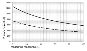
$\begin{array}{c} ---- U_{C} = \pm 24 \ V \ -5 \ \%, \ T_{A} = 85 \ ^{\circ}C \\ ---- U_{C} = \pm 15 \ V \ -5 \ \%, \ T_{A} = 85 \ ^{\circ}C \\ Primary currents higher than I_{PM} only for peak! \end{array}$
