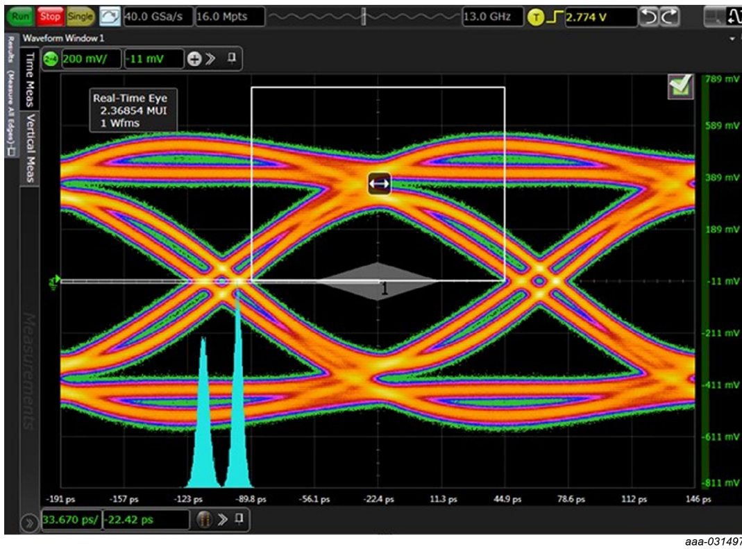
Fig. 9. HDMI 2.1 6 Gbps TMDS eye diagram, PCB with device; typical values
