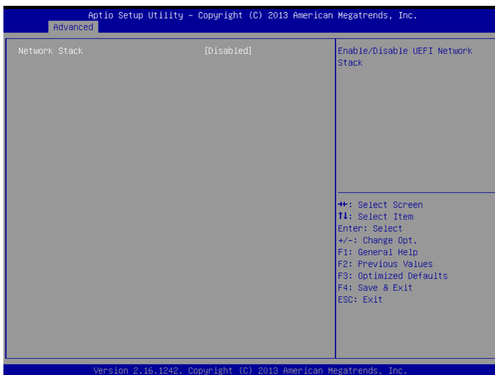
Figure 3.19 Network Stack Configuration
