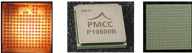
Figure 2. The ASIC chip and the BGA package.
