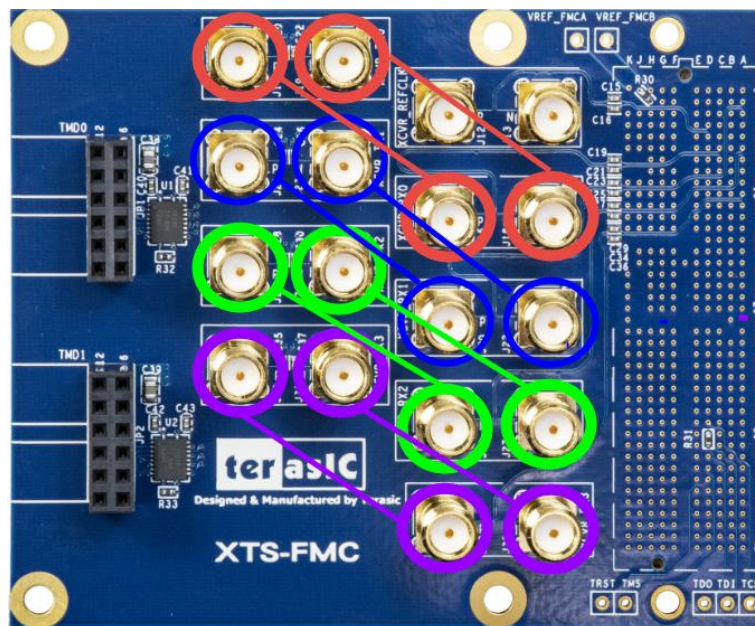
Figure 4-1 SMA loopback setup
