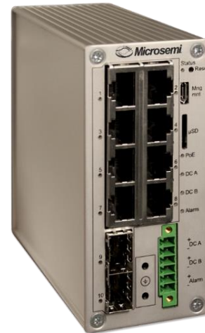
Industrial Ethernet Switch Reference Design Using VSC7514 Ocelot-10 Switch IC and IStAX Software
