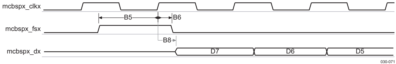
Figure 6-36. McBSP Rising Edge Transmit Timing in Slave Mode
