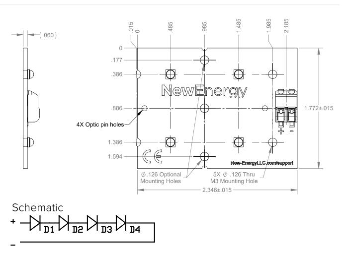
1. Dual Poke-In Connectors accept 18-24 AWG solid or stranded wire
