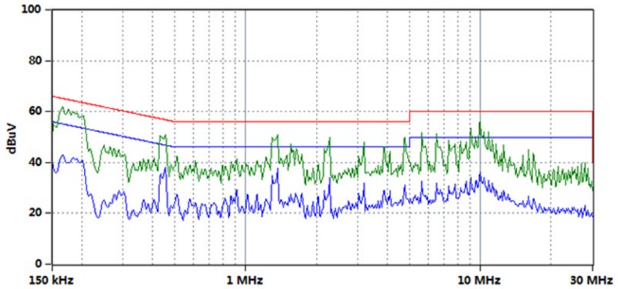
Fig. 11a: Conducted EMI (Quasi-Peak green/red and AVG blue/blue, V_{in} = 230 VAC, P_{out} = 150 W)
