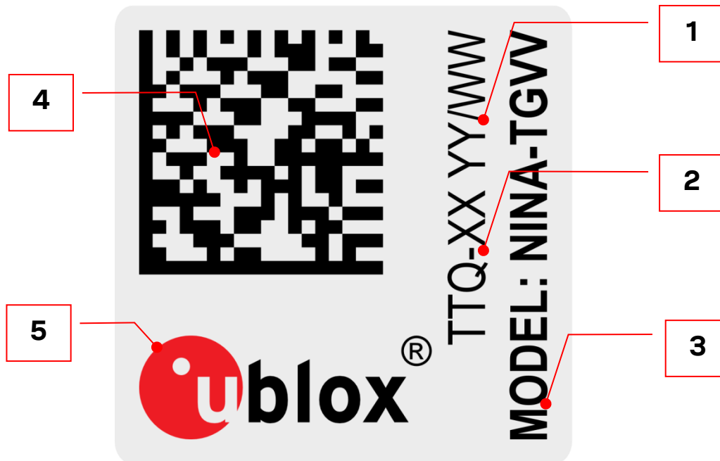
Figure 15: Location of product type number on the NINA-W13 series module label
