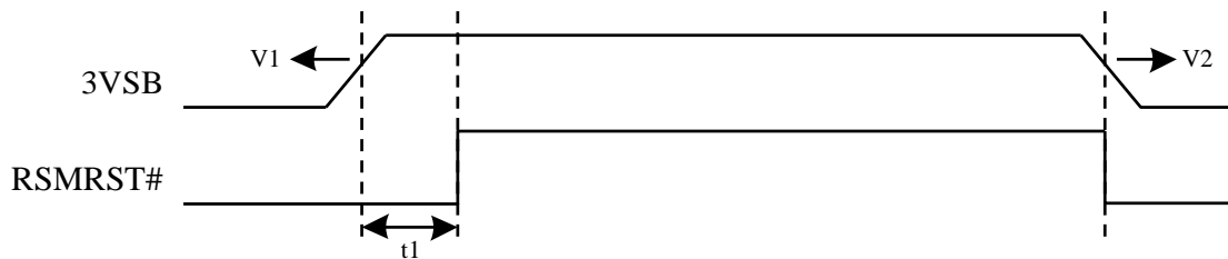
Figure 14-5 Mechanism of Resume Reset Logic
