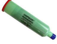
**Specifications** Alloy: Sn96.5/Ag3.0/Cu0.5 Mesh Size: T5 Micron (µm) Range: 15-25 Flux Type: Synthetic No-Clean Flux Classification: ROL0 Metal Load: 85.75% Metal by Weight Melting Point: 217-220°C (423-428°F) Packaging: 500g Cartridge Shelf Life: Refrigerated >6 months, Unrefrigerated >2 months \*See notes below:
