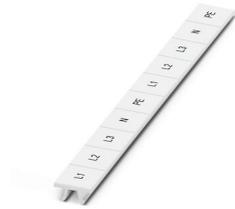
Marker for terminal blocks, Strip, white, labeled, can be labeled with: CMS-P1-PLOTTER, horizontal: L1, L2, L3, N, PE, L1, L2, L3, N, PE, mounting type: snapped, for terminal block width: 10.2 mm, lettering field size: 10,15 x 10,5 mm, Number of individual labels: 10
