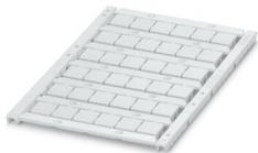
Marker for terminal blocks, can be ordered: by sheet, white, labeled according to customer specifications, mounting type: snap into tall marker groove, for terminal block width: 10.2 mm, lettering field size: 8.9 x 9.6 mm, Number of individual labels: 36
