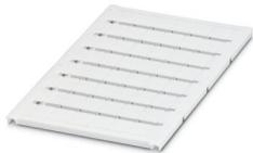
Marker for terminal blocks, can be ordered: by sheet, white, labeled according to customer specifications, mounting type: snap into tall marker groove, for terminal block width: 10.2 mm, lettering field size: 9.6 x 10.5 mm, Number of individual labels: 48
