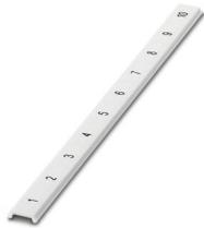
Zack Marker strip, flat, Strip, white, labeled, printed horizontally: consecutive numbers 1 ... 10, 11 ... 20, etc. up to 91 ... 100, mounting type: snapped, for terminal block width: 10 mm, lettering field size: 5.15 x 10 mm, Number of individual labels: 10
