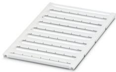
Marker for terminal blocks, Sheet, white, unlabeled, can be labeled with: BLUEMARK ID COLOR, BLUEMARK ID, BLUEMARK CLED, PLOTMARK, CMS-P1-PLOTTER, mounting type: snapped, for terminal block width: 10.2 mm, lettering field size: 9.6 x 5.1 mm, Number of individual labels: 48
