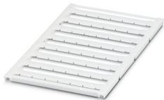
Marker for terminal blocks, can be ordered: by sheet, white, labeled according to customer specifications, mounting type: snap into flat marker groove, for terminal block width: 10.2 mm, lettering field size: 9.6 x 5.1 mm, Number of individual labels: 48
