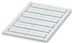
Marker for terminal blocks, Sheet, white, unlabeled, can be labeled with: TOPMARK NEO, TOPMARK LASER, BLUEMARK ID COLOR, BLUEMARK ID, BLUEMARK CLED, THERMOMARK PRIME, THERMOMARK CARD 2.0, THERMOMARK CARD, mounting type: snapped, for terminal block width: 10.2 mm, lettering field size: 9.4 x 4.7 mm, Number of individual labels: 36
