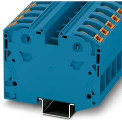
High-current terminal block, nom. voltage: 1000 V, nominal current: 125 A, number of connections: 2, connection method: PowerTurn connection, Rated cross section: 35 mm<sup>2</sup>, cross section: 2.5 mm<sup>2</sup> - 35 mm<sup>2</sup>, mounting type: NS 35/15, color: blue
