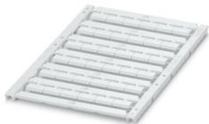
Marker for terminal blocks, can be ordered: by sheet, white, labeled according to customer specifications, mounting type: snap into flat marker groove, for terminal block width: 10.2 mm, lettering field size: 9.4 x 4.7 mm, Number of individual labels: 36
