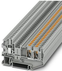
Feed-through terminal block, nom. voltage: 800 V, nominal current: 32 A, connection method: Push-in connection, Rated cross section: 4 mm<sup>2</sup>, cross section: 0.2 mm<sup>2</sup> - 6 mm<sup>2</sup>, connection method: Screw connection, Rated cross section: 4 mm<sup>2</sup>, cross section: 0.14 mm<sup>2</sup> - 6 mm<sup>2</sup>, mounting: NS 35/7,5, NS 35/15, color: gray
