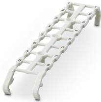
Marker for terminal blocks, white, labeled, mounting type: snapped, for terminal block width: 8 mm, lettering field size: 2.4 x 9.2 mm, Number of individual labels: 2
