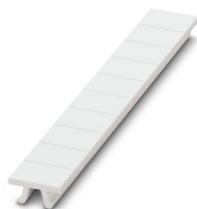
Zack marker strip, Strip, white, labeled according to customer specifications, mounting type: snap into tall marker groove, for terminal block width: 8.3 mm, lettering field size: 10.5 x 8.3 mm
