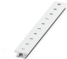
Zack marker strip, Strip, white, labeled, can be labeled with: CMS-P1-PLOTTER, mounting type: snapped, for terminal block width: 8.3 mm, lettering field size: 10.5 x 8.3 mm
