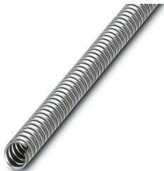
Protective hose, material: Stainless steel 1.4301/AISI 304, degree of protection: IP40, color: silver, inner diameter: 11 mm, Total length: 10 m
