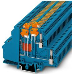
Knife-disconnect terminal block, With test socket screws for insertion of test plugs, nom. voltage: 400 V, nominal current: 10 A, 1st and 2nd level, connection method: Screw connection, Rated cross section: 4 mm<sup>2</sup>, cross section: 0.2 mm<sup>2</sup> - 4 mm<sup>2</sup>, 2nd level, connection method: Screw connection, Rated cross section: 4 mm<sup>2</sup>, cross section: 0.2 mm<sup>2</sup> - 4 mm<sup>2</sup>, mounting: NS 35/7,5, NS 35/15, NS 32, color: blue
