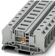
Test disconnect terminal block, Note: the BE-RT... path extension is to be used for non-insulated cable lugs (see accessories)., nom. voltage: 1000 V, nominal current: 41 A, 1 level, connection method: Bolt connection, Rated cross section: 6 mm<sup>2</sup>, mounting: NS 35/7,5, NS 35/15, color: gray
