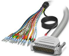
Assembled shielded round cable; connection 1: Single wires (25-position) (The wires are marked and fitted with ferrules. The braided shield is routed to a separate cable end.); connection 2: D-SUB pin strip (1x 25-position); cable length: 0.5 m
