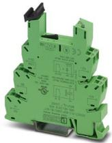
14 mm PLC basic terminal block for high switch-on currents with spring-cage connection, without relay or solid-state relay, for mounting on DIN rail NS 35/7,5, with load return line connection (BB), 1 N/O contact, input voltage 24 V DC
