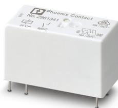
Pluggable miniature power relay, with power contact for high switch-on currents up to 130 A peaks, 1 N/O contact, input voltage: 24 V DC
