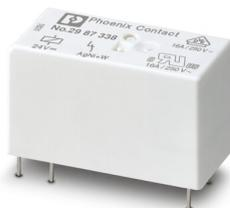
Pluggable miniature power relay, with tungsten pre-contact for high switch-on currents up to 800 A peaks, 1 N/O contact, input voltage: 24 V DC
