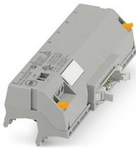
V8 adapter for 8 x PLC-INTERFACE (14 mm), controller: PLC system cabling of output cards, connection 1: IDC/FLK pin strip 1x 14-position, connection 2: Plug-in connection (Can be snapped onto 8x PLC-INTERFACE terminals), connection 3: Screw connection 1x 2-position, number of channels: 8, control logic: minusschaltend
