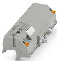
V8 adapter for 8 x PLC-INTERFACE (14 mm), controller: PLC system cabling of output cards, connection 1: IDC/FLK pin strip 1x 14-position, connection 2: Plug-in connection (Can be snapped onto 8x PLC-INTERFACE terminals), connection 3: Screw connection 1x 2-position, number of channels: 8, control logic: plusschaltend
