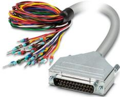
Assembled shielded round cable; connection 1: Twisted pair (25-position) (The wires are marked and fitted with ferrules); connection 2: D-SUB pin strip (1x 25-position); cable length: 3 m
