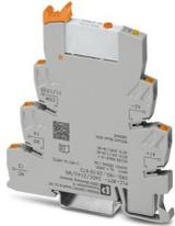
PLC-INTERFACE, consisting of PLC-BPT.../21 basic terminal block with Push-in connection and plug-in miniature relay with multi-layer gold contact and manual operation, 1 changeover contact, 24 V DC input voltage
