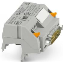
V8 adapter for 8 x PLC-INTERFACE (6.2 mm), controller: PLC system cabling of input cards, connection 1: D-SUB pin strip 1x 15-position, connection 2: Plug-in connection (Can be snapped onto 8x PLC-INTERFACE terminals), connection 3: Screw connection 1x 2-position, number of channels: 8, control logic: plusschaltend
