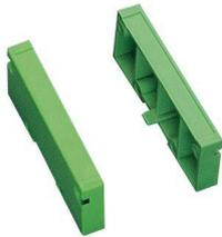
Press-drawn section housings, Lateral element, color: green (6021), without snap-on foot, depth: 45 mm, Note: when using this lateral element, profile length = PCB length.
