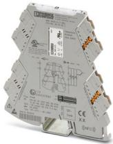
Universally configurable temperature limit value switch with N/O relay output for the connection of 2, 3, and 4-conductor resistance thermometers and thermocouples. Configurable via DIP switch or software, screw connection technology
