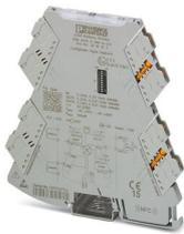
Universally configurable 4-way signal duplicator, with plug-in connection technology for the electrical isolation and duplication of analog signals. Configurable via DIP switch or software. Screw connection technology, standard configuration.
