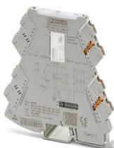
Universally configurable temperature limit value switch with N/O relay output for the connection of 2, 3, and 4-conductor resistance thermometers and thermocouples. Configurable via DIP switch or software. Push-in connection technology
