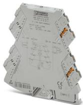
3-way signal conditioner with plug-in connection technology for the electrical isolation of analog signals. Input signal: 0 V ... 10 V, output signal: 0 mA ... 20 mA, push-in connection technology
