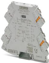
Configurable NAMUR signal conditioner with plug-in connection technology for proximity sensors, floating switch contacts, and switch contacts with resistance circuit. 2 transistor outputs. Configurable via DIP switch. Push-in connection technology.
