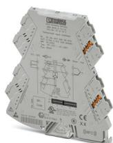
Configurable temperature transducer with plug-in connection technology for connecting thermocouples. Configurable via DIP switch or software. Screw connection technology, standard configuration
