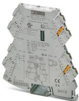
Universally configurable 4-way signal conditioner, with switching output and plug-in connection technology for the electrical isolation of analog signals. Configurable via DIP switch or software. Push-in connection technology, order configuration.
