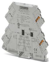
3-way signal conditioner with plug-in connection technology and calibrated measuring range changeover for the electrical isolation of unipolar and bipolar analog signals. Input/output configurable via DIP switch. push-in connection technology, order configuration.
