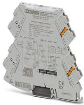
Universally configurable frequency transducer for converting frequency (Hz/rpm) and PWM signals into standard signals. Sensor voltages greater than 8.2 V DC are possible in combination with MINI MCR-2-SPS-PT 1033201. Push-in connection technology.
