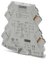
Configurable potiposition transducer with plug-in connection technology for connecting potentiometers from 0  $\Omega$  ... 100  $\Omega$  to 0 k $\Omega$  ... 100 k $\Omega$ . Configurable via DIP switch or software. Screw connection technology, standard configuration
