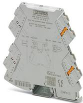
1-channel input loop-powered 2-way isolator with plug-in connection technology for the electrical isolation of analog signals. Input signal = output signal: 0(4) mA ... 20 mA. Push-in connection technology.
