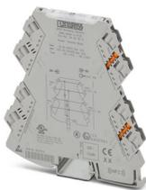
Power terminal with plug-in connection technology for delivering the supply voltage to the DIN rail connector. Monitoring of the supply voltages in combination with the fault monitoring module. Screw connection technology
