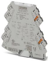
3-way repeater power supply with plug-in connection technology. HART-transparent, input signal 0(4)...20 mA, output signal 0(4)...20 mA. The device can be used in both isolator and repeater power supply operation. Screw connection technology
