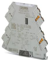
Universally configurable 4-way signal duplicator, with plug-in connection technology for the electrical isolation and duplication of analog signals. Configurable via DIP switch or software. Push-in connection technology, order configuration.
