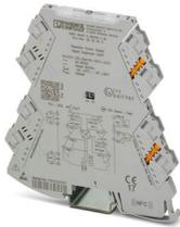
4-way power supply doubler with plug-in connection technology. HART-transparent, 0(4) mA ... 20 mA input signal, 0(4) mA ... 20 mA output signals. The device can be used in both signal and power supply doubler modes. Screw connection technology.
