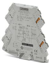
Configurable temperature transducer with plug-in connection technology for connecting 2, 3, and 4-conductor resistance thermometers and resistance-type sensors. Configurable via DIP switch or software. push-in connection technology, order configuration
