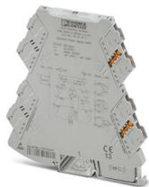
3-way repeater power supply with plug-in connection technology. HART-transparent, input signal 0(4) mA ... 20 mA, output signal 0(4) mA ... 20 mA. The device can be used in both isolator and repeater power supply operation. push-in connection technology
