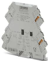
3-way signal conditioner with plug-in connection technology and calibrated measuring range changeover, for the electrical isolation of unipolar and bipolar analog signals. Input/output configurable via DIP switch. push-in connection technology, standard configuration.
