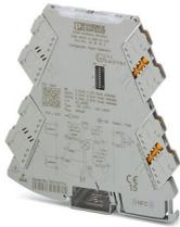
Universally configurable 4-way signal duplicator, with plug-in connection technology for the electrical isolation and duplication of analog signals. Configurable via DIP switch or software. Screw connection technology, order configuration.
