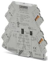
3-way signal conditioner with plug-in connection technology and calibrated measuring range changeover for the electrical isolation of unipolar and bipolar analog signals. Input/output configurable via DIP switch. Screw connection technology, standard configuration.
