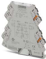
3-way signal conditioner with plug-in connection technology for the electrical isolation of analog signals. Input signal: 0 V ... 10 V, output signal: 0 mA ... 20 mA, screw connection technology
