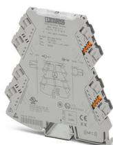
3-way signal conditioner with plug-in connection technology for the electrical isolation of analog signals. Input signal: 0(4) mA ... 20 mA, output signal: 0(4) mA ... 20 mA, screw connection technology
