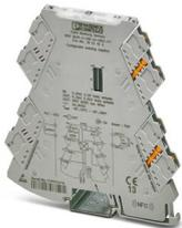
Universally configurable 4-way signal conditioner, with switching output and plug-in connection technology for the electrical isolation of analog signals. Configurable via DIP switch or software. Push-in connection technology, standard configuration.
