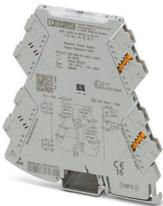
4-way power supply doubler with plug-in connection technology. HART-transparent, 0(4) mA ... 20 mA input signal, 0(4) mA ... 20 mA output signals. The device can be used in both signal and power supply doubler modes. Push-in connection technology.
