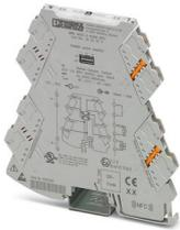
Configurable NAMUR signal conditioner with plug-in connection technology for proximity sensors, floating switch contacts, and switch contacts with resistance circuit. 2 transistor outputs, configurable via DIP switch. Screw connection technology.
