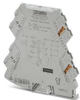
Configurable potiposition transducer with plug-in connection technology for connecting potentiometers from 0  $\Omega$  ... 100  $\Omega$  to 0 k $\Omega$  ... 100 k $\Omega$ . Configurable via DIP switch or software. push-in connection technology, standard configuration
