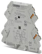
Fault monitoring module with plug-in connection technology for evaluating and reporting group errors from the FM system and for monitoring the supply voltages. Error message via N/C contact. Push-in connection technology, standard configuration
