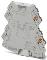
1-channel input loop-powered 2-way isolator with plug-in connection technology for the electrical isolation of analog signals. Input signal = output signal: 0(4) mA ... 20 mA. Screw connection technology.
