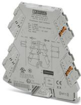
Configurable potiposition transducer with plug-in connection technology for connecting potentiometers from 0  $\Omega$  ... 100  $\Omega$  to 0 k $\Omega$  ... 100 k $\Omega$ . Configurable via DIP switch or software. Screw connection technology, order configuration
