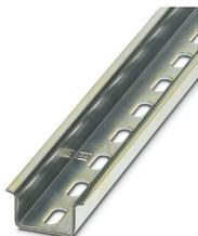
DIN rail perforated, similar to EN 60715, material: Steel, galvanized, passivated with a thick layer, Standard profile, color: silver, Pack of 25 (50 m)
