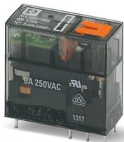
Plug-in miniature relay, with power contact, 2 changeover contacts, test button, mechanical switching position indicator, status LED, coil voltage 120 V AC
