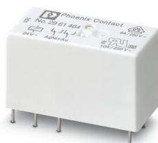
Plug-in miniature power relay, with multi-layer gold contact, 2 changeover contacts, input voltage 24 V AC
