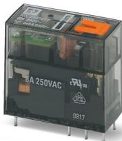
Plug-in miniature relay, with power contact, 2 changeover contacts, test button, mechanical switching position indicator, status LED, coil voltage 230 V AC
