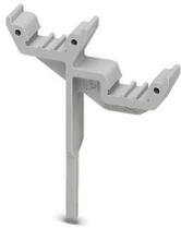
Marker carriers, snaps into STTB 2,5, STTB 4, PTTB 2,5, and PTTB 4 double-level spring-cage terminal blocks, can be marked with UC-TM 5, UC-TMF 5, UCT-TM 5, UCT-TMF 5, ZB 5, or ZBF 5, gray, unlabeled, mounting type: plug in, lettering field size: 5 x 10.5 mm
