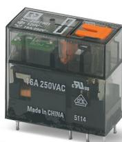
Plug-in miniature relay, with power contact, 1 changeover contact, test button, mechanical switching position indicator, status LED, input voltage 120 V AC
