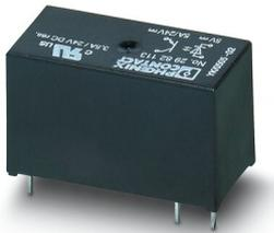
Plug-in miniature solid-state relay, power solid-state relay, 1 N/O contact, input: 5 V DC, output: 3 - 33 V DC/5 A
