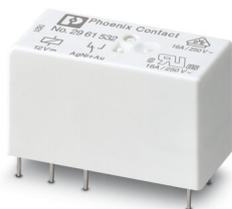
Plug-in miniature power relay, with multi-layer gold contact for high continuous currents, 1 changeover contact, input voltage 12 V DC
