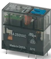
Plug-in miniature relay, with multi-layer contact with hard gold coating, 1 changeover contact, test button, mechanical switching position indicator, status LED, freewheeling diode, polarity A1+, A2-, input voltage 24 V DC
