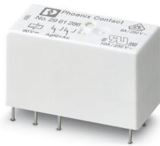
Plug-in miniature power relay, with multi-layer gold contact, 2 changeover contacts, input voltage 60 V DC
