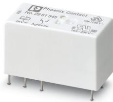
Plug-in miniature power relay, with multi-layer gold contact for high continuous currents, 1 changeover contact, input voltage 24 V DC
