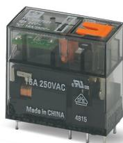
Plug-in miniature relay, with power contact, 1 changeover contact, test button, mechanical switching position indicator, status LED, input voltage 24 V AC
