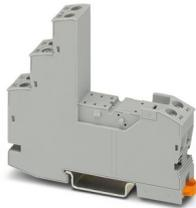
RIF-1... relay base, for miniature power relay with 1 or 2 changeover contacts or identical solid-state relays, screw connection, plug-in option for input/interference suppression modules, for mounting on NS 35/7,5
