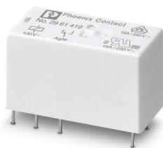
Plug-in miniature power relay, with power contact for high continuous currents, 1 changeover contact, input voltage 120 V AC
