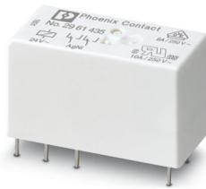
Plug-in miniature power relay, with power contact, 2 changeover contacts, input voltage 24 V AC
