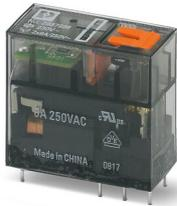
Plug-in miniature relay, with multi-layer contact with hard gold coating, 2 changeover contacts, test button, mechanical switching position indicator, status LED, coil voltage 230 V AC
