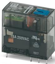
Plug-in miniature relay, with power contact, 1 changeover contact, test button, mechanical switching position indicator, status LED, freewheeling diode, polarity A1+, A2-, input voltage 24 V DC
