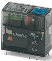
Plug-in miniature relay, with power contact, 2 changeover contacts, test button, mechanical switching position indicator, status LED, freewheeling diode, polarity A1+, A2, input voltage 24 V DC
