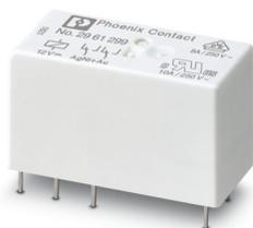
Plug-in miniature power relay, with multi-layer gold contact, 2 changeover contacts, input voltage 12 V DC
