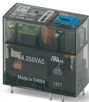
Plug-in miniature relay, with multi-layer contact with hard gold coating, 2 changeover contacts, test button, mechanical switching position indicator, status LED, freewheeling diode, polarity A1+, A2-, input voltage 24 V DC
