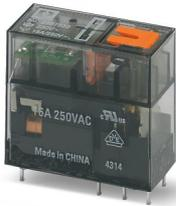
Plug-in miniature relay, with multi-layer contact with hard gold coating, 1 changeover contact, test button, mechanical switching position indicator, status LED, input voltage 230 V AC
