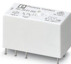
Plug-in miniature power relay, with power contact, 2 changeover contacts, input voltage 110 V DC
