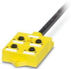
The sensor box PSR-SACB for safety limit switches safely interconnects up to 4 connected limit switches, each with 1 N/C contact and 1 N/O contact, to a safety relay combination, e.g. PSR-SDC4, cable length: 5 m
