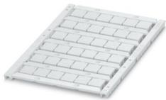
Marker for terminal blocks, Sheet, white, unlabeled, can be labeled with: TOPMARK NEO, TOPMARK LASER, BLUEMARK ID COLOR, BLUEMARK ID, BLUEMARK CLED, THERMOMARK PRIME, THERMOMARK CARD 2.0, THERMOMARK CARD, mounting type: snapped, for terminal block width: 10.2 mm, lettering field size: 8.9 x 9.6 mm, Number of individual labels: 36
