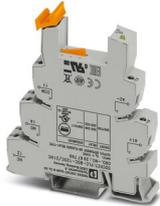
14 mm PLC basic terminal block for high continuous currents with screw connection, without relay or solid-state relay, for mounting on DIN rail NS 35/7,5, 1 changeover contact, input voltage 12 V DC
