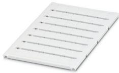
Marker for terminal blocks, can be ordered: by sheet, white, labeled according to customer specifications, mounting type: snap into tall marker groove, for terminal block width: 12 mm, lettering field size: 11.45 x 10.5 mm, Number of individual labels: 40
