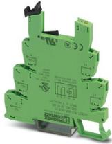
6.2 mm PLC basic terminal block with spring-cage connection, without relay or solid-state relay, for mounting on DIN rail NS 35/7,5, 1 changeover contact, input voltage 24 V AC/DC
