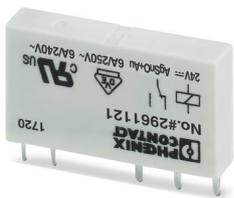
Plug-in miniature power relay, with multi-layer gold contact, 1 changeover contact, input voltage 24 V DC
