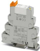
PLC-INTERFACE for output functions, consisting of PLC-BSC.../ACT basic terminal block with screw connection and plug-in miniature relay with power contact, for mounting on DIN rail NS 35/7,5, 2 N/O contacts (1-1), input voltage 24 V DC
