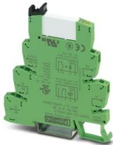
PLC-INTERFACE, consisting of PLC-BSP.../21 basic terminal block with spring-cage connection and plug-in miniature relay with multi-layer gold contact, for mounting on DIN rail NS 35/7,5, 1 changeover contact, input voltage 230 V AC/220 V DC
