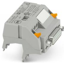
V8 adapter for 8 x PLC-INTERFACE (6.2 mm), controller: PLC system cabling of input cards, connection 1: D-SUB socket strip 1x 15-position, connection 2: Plug-in connection (Can be snapped onto 8x PLC-INTERFACE terminals), connection 3: Screw connection 1x 2-position, number of channels: 8, control logic: plusschaltend
