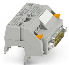
V8 adapter for 8 x PLC-INTERFACE (6.2 mm), controller: PLC system cabling of input cards, connection 1: D-SUB pin strip 1x 15-position, connection 2: Plug-in connection (Can be snapped onto 8x PLC-INTERFACE terminals), connection 3: Screw connection 1x 2-position, number of channels: 8, control logic: plusschaltend
