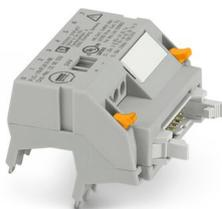
V8 adapter for 8 x PLC-INTERFACE (6.2 mm), controller: PLC system cabling of input cards, connection 1: IDC/FLK pin strip 1x 14-position, connection 2: Plug-in connection (Can be snapped onto 8x PLC-INTERFACE terminals), connection 3: Screw connection 1x 2-position, number of channels: 8, control logic: plusschaltend
